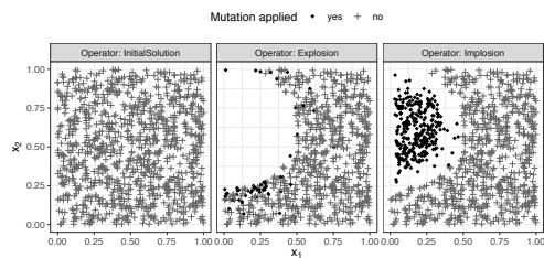
Figure 4: Explosion and implosion operators.
